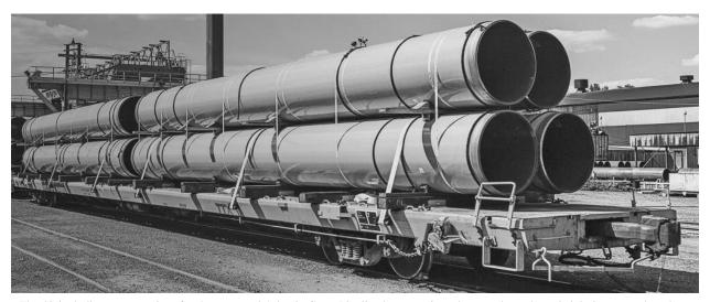
The 42-inch diameter gas pipes for the proposed Atlantic Coast Pipeline have coatings that may have degraded during more than three years of exposure after transport. (File photo)
