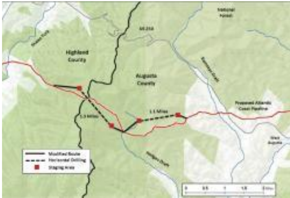
Rick Webb’s map of the proposed horizontal drill through Shenandoah Mountain depicts an approximate route, based on Dominion’s comments. The red squares depict possible horizontal drilling staging areas. The dashed lines are possibly drilled sections.
